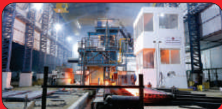
Continuous Casting Machine
