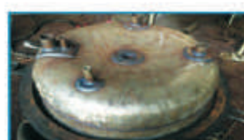
Gas Carburising Furnace
