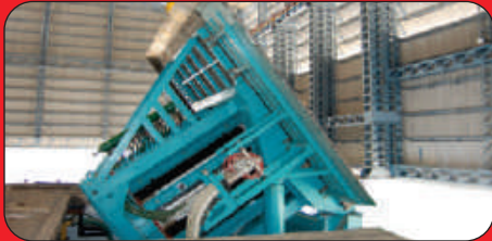
Induction Melting Furnace
