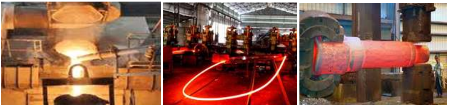
Steel Melting in IF, Rolling in Re-Rollin Mill, Forging in Forging Press ,
