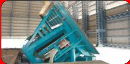
Induction Melting Furnace
