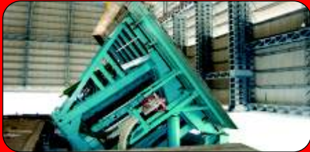
Induction Melting Furnace
