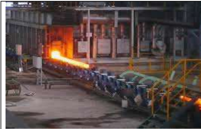
Billet Re-Heating Fce. in Re-Rolling Mill
