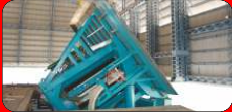
Induction Melting Furnace
