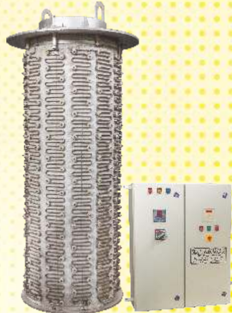
Ladle and Sintering Preheater with Bottom Heater
